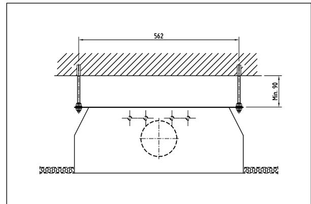
Figure 7. Polaris I 60 recessed in a suspended ceiling.
